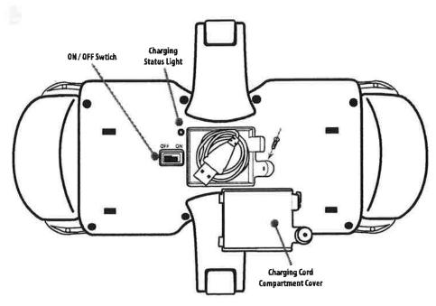
This vehicle is equipped with an internal Lithium-Ion battery that is recharged via USB.
