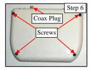
Finally, attach the dipole antenna to the coaxial cable plug by placing the antenna over the plug and screwing in a clockwise direction. The antenna is sufficiently secured when it is flush with the HUB enclosure.
