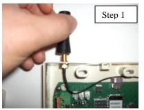
**Step 1:** Identify the *Antenna, helical short ¼ wave* (A). Screw the antenna into the gold coaxial antenna connector on the top of the *IREP assembly* (B). Ensure that the antenna is screwed onto the connector snugly, but take care not to over-tighten the antenna as it will damage the connector or the IREP assembly enclosure.
