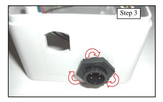
**Step 4:** Take the bulkhead RF cable (F) and remove the nut and washer. Insert the bulkhead into the inside of the front enclosure with the pin facing out. Fasten the washer to the bulkhead (outside of the enclosure) and rotate the nut clockwise until it is flush against the bottom enclosure.
