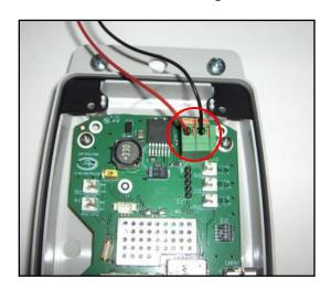
**Step 6:** Insert the pigtail connector end of the RF cable into the RF port labeled J1 on the PCB by laying connector over the port and pressing down on the connector. The connector should snap right into place.
