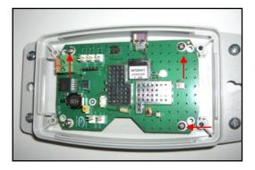
**Step 2:** Identify the rubber mat and line the holes up with the elevated screw holes in each corner. Feed the openings on the rubber mat through the double pegs beside each elevated screw hole.
