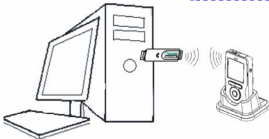
Figure 3-2: Install wireless USB Dongle
