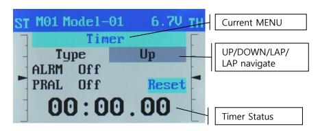
Select TYPE first and select the type of timer using the UP/DOWN.
