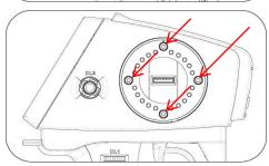
7. Screw in the 4 screws on the wheel holder. These screws are separately provided.
