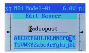
Move to the character to be input using the direction buttons (**LEFT/RIGHT/UP/DOWN**) and press the **SET**. Change the other characters in the other positions in the same way.
