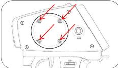
2. Detach the empty wheel cover on the left side of transmitter by taking off the 4 screws and attach it to the right side.
