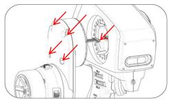
1. Take off the 4 screws on the adapter neck and disconnect the wire.
