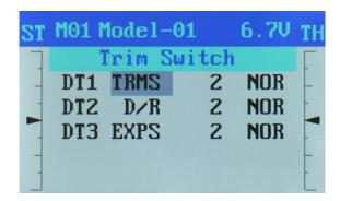
All the functions for the dial switches as shown in the table of the Dial Switch section can be assigned to the trim switches.
