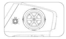
11. Assemble the wheel by driving the center screw.
