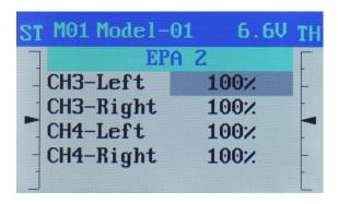
Use the "CH3-LEFT" to set the maximum left end point of 3<sup>rd</sup> channel. Use the "CH3-RIGHT" to set the maximum right end point of 3<sup>rd</sup> channel. Use the "CH4-LEFT" to set the maximum left end point of 4<sup>th</sup> channel. Use the "CH4-RIGHT" to set the maximum right end point of 4<sup>th</sup> channel. The maximum end point has an adjustable range from 50% to 120% and default value is 100%.
