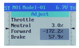
Press the **SET** to save the neutral position value, the Forward maximum value and the Brake maximum value.
