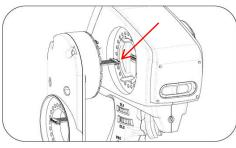
5. Detach the adapter from the transmitter body and disconnect the wire.
