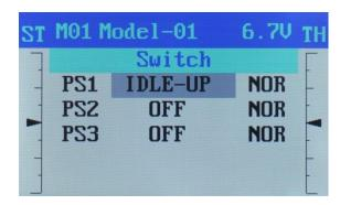
The table shows the functions that can be assigned to the push switches.
