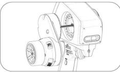
2. Pull the adapter softly and adjust the wheel angle to the desired direction. The angle can be adjusted by every 15°.
