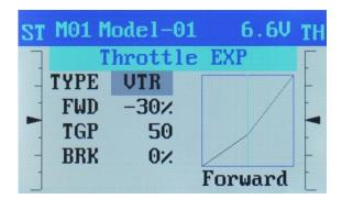
CRV: Press the SET on TYPE and select CRV. Press the DOWN to move to FWD.
