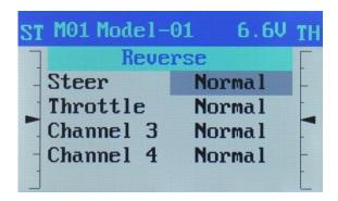
Move to the preferred channel by using the **UP/DOWN** and press the **SET**. Press the **LEFT** or **RIGHT** to select Normal or Reverse. Press the **SET** to save the adjusted value.
