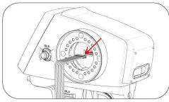
8. Plug in the wire to the transmitter body. Use the wire which is provided separately.
