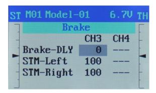
Move to the Brake-DLY in the next page by pressing the **DOWN** on Brake-EXP. Press the **SET** on Brake-DLY to set the brake delay time. The brake delay time can be set to the front or rear brake.
