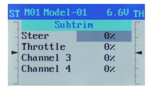
Adjust the Servo movement with the Steer channel so that the steering can be in a neutral position. The available setting range is from L 100%(left) to R 100% (right). Use the "Throttle channel" to make the servo control the engine throttle at neutral. The available setting range is from F 100% (accelerator) to B 100% (brake). The aux channels (channel 3 and 4) have the available settings ranging from -100% to 100%. The default value is 0%.
