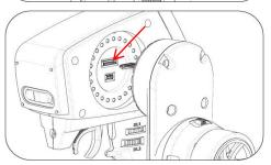
3. Connect the wire to the transmitter body.
