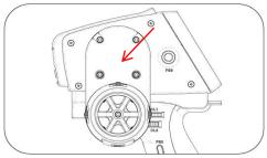
4. Connect the adapter for wheel extension by driving the 4 screws.
