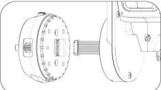
3. Separate the wheel set from the adapter and disconnect the wire.
