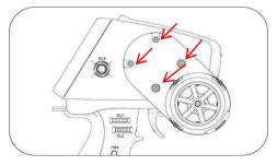
3. Mount the adapter to the transmitter body keeping the adjusted angle and drive the 4 screws on the adapter neck.
