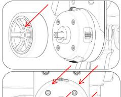
1. Detach the wheel by first taking off the screw at the center of steering wheel using the hex wrench.
