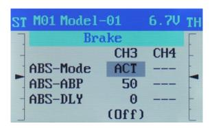
Move to the ABS-ABP using the **DOWN** to set the brake return amount value. The value range is 0 to 100. The default value is 50. When the value is 0, no brake return is carried out, which means ABS function does not work. When the value is 50, the brake return is carried out to the 50% position of trigger point. When the value is 100, the brake servo performs the brake return to the neutral position.
