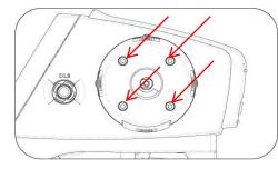
10. Screw in the 4 screws on the wheel set. Use the screws which were taken off in the Step 2.
