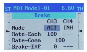
Move to the RATE-EACH using the **DOWN** to set the mixing ratio. The range of mixing ratio is 0 to 100. The default value is 100.
