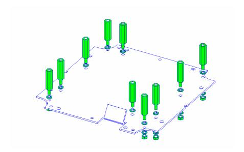
Attach the lower **board** into the **front box** and assemble **screws**.
