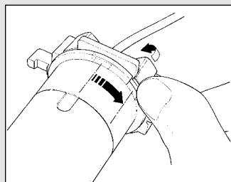
Rotate the ring nut until the chamfer matches one of the latch-on teeth.
