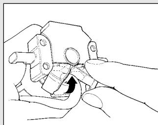
Bend the cable inward and remove the protection by rotating it gently outward.
