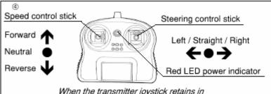
When the transmitter joystick retains in its neutral position, the power of the transmitter is automatically cut off.
