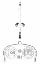
Do not install the antenna extended.
