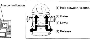
\* The robot will repeat these four movements while the button is held pressed.
