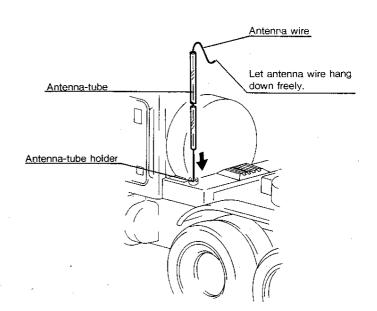
\* Pass antenna wire through antenna tube and insert the antenna tube into antenna tube holder.
