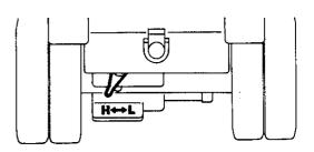
\*If the selector switch (gear shift) should not move smoothly, slight turning of the rear wheels by hand will facilitate shifting.
