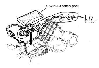
Disconnect the connectors as shown after a run.
