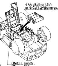
Let the battery compartment lid slide forward a littlee with a pressure on to the latch. Then, the battery compartment lid can be pulled and open.
