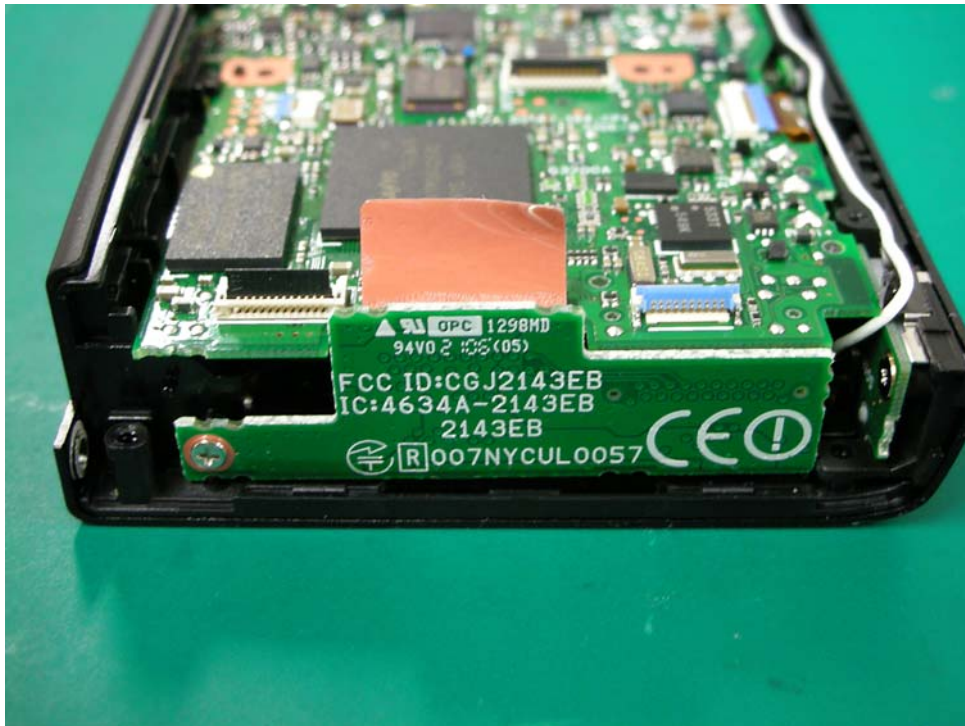
Fig3. Side view of “2143EB” be equipped for a digital camera (example)
