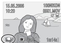
To play a movie, display it in full-frame playback and press the **OK** button. Playback controls appear at the top of the display; press the rotary multi selector left or right to highlight a control, then press the **OK** button to perform the selected operation.
