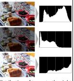
Exposure compensation shifts the distribution of tones to the right when raised, to the left when lowered. Histograms can give you a rough idea of overall exposure when bright ambient lighting makes it difficult to see the display in the monitor.
