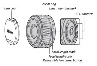
1 NIKKOR lenses are exclusively for Nikon 1 interchangeable lens format digital cameras. The angle of view is equivalent to a 35 mm format lens with a focal length about 2.7× longer. The 1 NIKKOR VR 10–30mm f/3.5–5.6 supports normal and active vibration reduction and vibration reduction off ( $\Box$  127).
