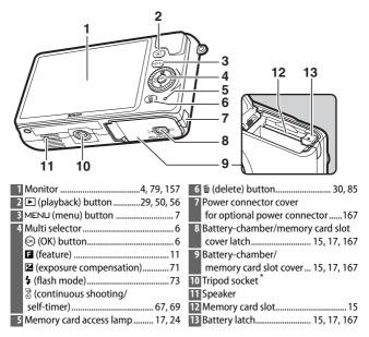
\*Camera does not support TA-N100 tripod mounting spacer.
