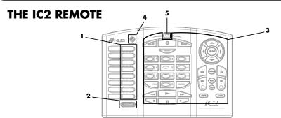
Figure 1. iC2 Remote Front View
