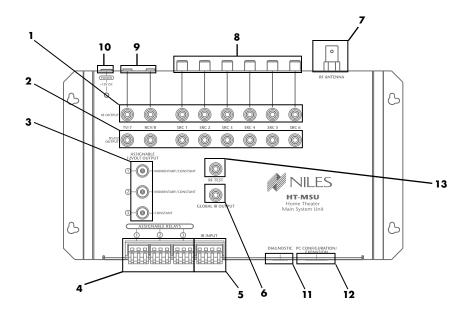
Figure 4. HT-MSU Top View
