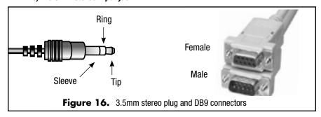
Most sources that are RS232 controllable provide a protocol document (usually from their Tech Support Department) that will have all of the necessary information, including pin-out, to custom build the RS232 control cable (**Figure 16**).
