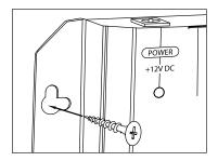
Figure 8. Wall-mount placement Use sheetrock screws
