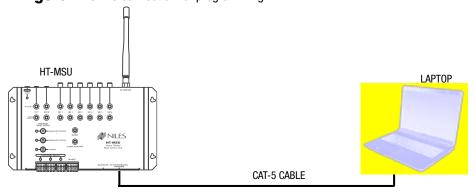
**Figure 12.** PC connection for programming when using optional RFG.
