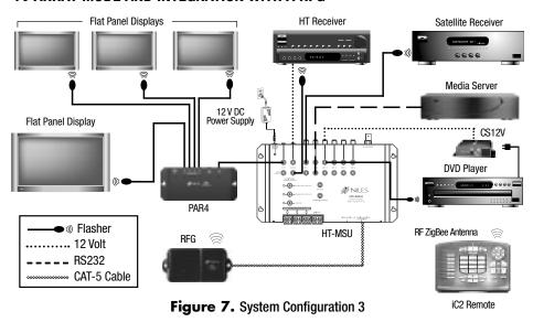
System Configuration #3 (**Figure 7**), shows two more system design features of the iC2 System. The iC2 System has a design feature called TV Array. Here, a Niles PAR4 Simplified IR Router is used with the HT-MSU to control an array of identical televisions.
