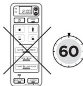
6. During 60-minute Clean Cycle, do not press any buttons. Unit may dim.
