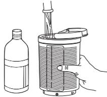
2. Fill reservoir to Max Fill line with descaling solution\* and water or white vinegar\*\* and water.
