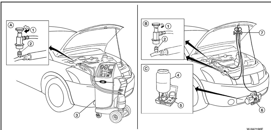
1. Shut-off valve                      2. A/C service valve                      3. Recovery/recycling equipment
