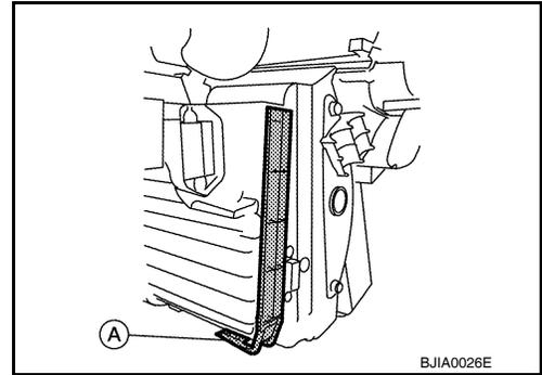
2. Remove the in-cabin microfilter.
