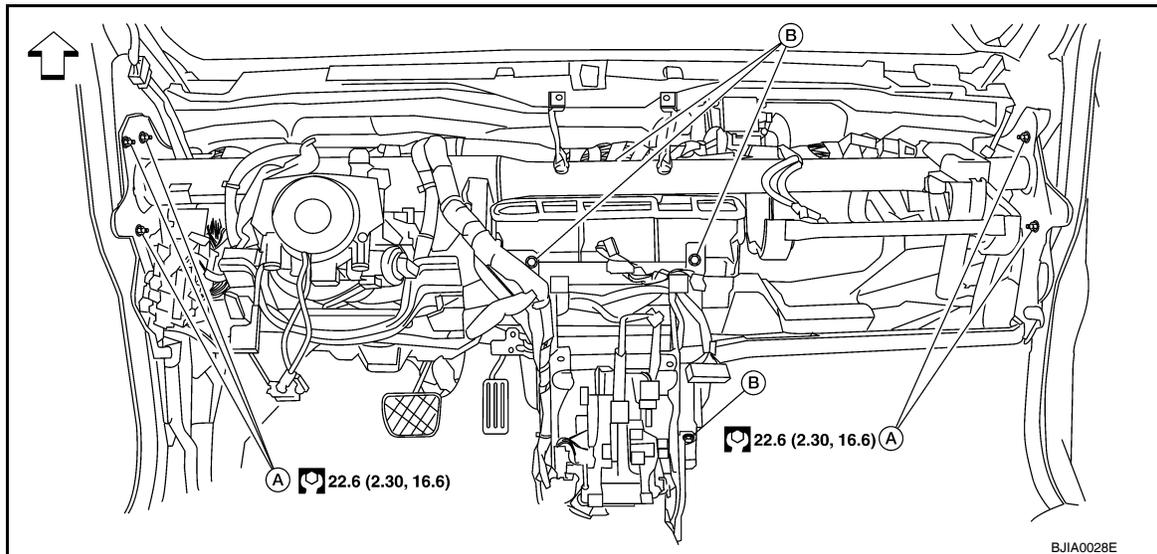
A. Steering member bolts      B. Heater and cooling unit assembly bolts      ← Vehicle front
