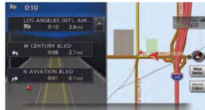
Depending on the setting, the system can constantly display the split screen and show the turn list on the left screen. When approaching a guide point, the left screen automatically switches to an enlarged view of the intersection. To switch to the full screen mode, push **<MAP>**. Pushing **<MAP>** again displays the turn list.
