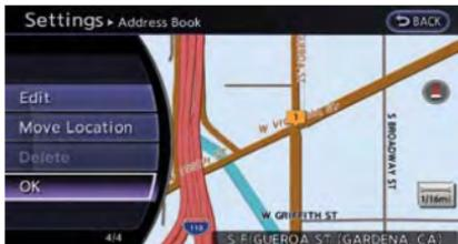
8. Adjust the location of the stored item and edit the contents of the stored item as necessary. After finishing the setting, highlight [OK] and push **<ENTER>**.
