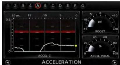
Displays the accelerator pedal position, boost pressure and the g-force being exerted on the vehicle.
