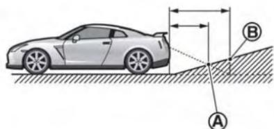
When backing up the vehicle up a hill, the distance guide lines and the vehicle width guide lines are shown closer than the actual distance. For example, the display shows 3 ft (1.0 m) to the place **(A)**, but the actual 3 ft (1.0 m) distance on the hill is the place **(B)**. Note that any object on the hill is further than it appears on
