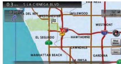
When route guidance starts, the Small Turn Arrow on Map is displayed in the upper left corner of the map screen. This arrow indicates the turning direction at the next guide point (corner or intersection). The distance is also displayed. At the top of the screen, the distance to the next guide point and the name of the next street to turn on to are displayed. Also, there may be cases that next street names are announced. The Small Turn Arrow on Map can be enabled or disabled by the user.
