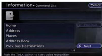
6. To confirm the list, scroll the screen using the up and down switches of the main directional buttons or the center dial.
