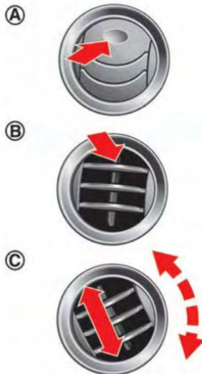
The direction of the air flow can be adjusted by **(A)** opening, **(B)** closing or **(C)** adjusting.
