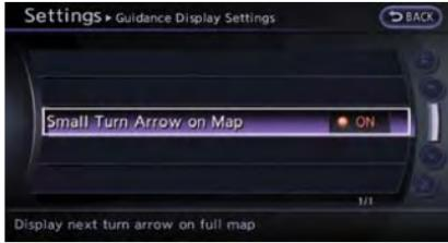
5. Highlight [Small Turn Arrow on Map] and push <ENTER> to activate or deactivate Small Turn Arrow on the Map (simplified turn indicator) displayed in the upper left corner of the map screen. The indicator illuminates if the Small Turn Arrow on the Map is displayed.
