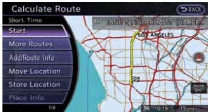
4. The entire route is shown on the map. Highlight [Start] after confirming the location of the displayed destination, and push <ENTER>. The system sets the destination to the selected location and starts calculating a route.
