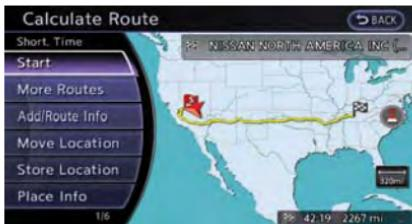
7. The entire route is shown on the map. Highlight [Start] after confirming the location of the displayed destination, and push <ENTER>. The system sets the destination to the selected location and starts calculat-
