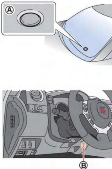
The sensors **(A)** and **(B)** on the instrument panel help maintain a constant temperature. Do not put anything on or around these sensors.
