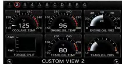
The driver can select up to six different meters to be displayed.
