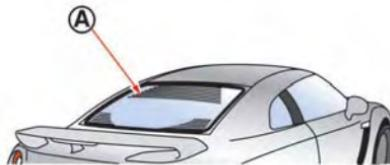
The antenna pattern is printed inside the rear window.
