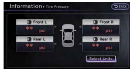
If there is a TPMS malfunction, the tire pressures are not displayed. The system displays "\*\*\*\*" instead of a pressure value.
