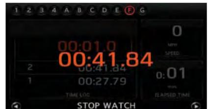
Displays the recorded driving time, vehicle speed and elapsed time and saves the history for each of these functions.
