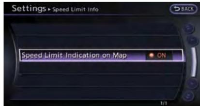
2. Highlight [Speed Limit Indication on Map] to toggle the function between on and off. The indicator light illuminates when the speed limit display function is set to on.
