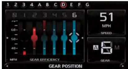
Displays the gear position, vehicle speed and each gear's fuel economy level/torque map.
