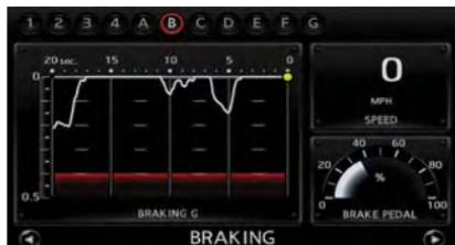
Displays the brake pedal position, vehicle speed and the g-force being exerted on the vehicle.
