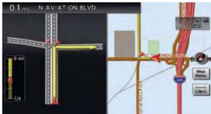
When approaching a guide point, the system automatically changes to the split screen and shows an enlarged view of the intersection on the left screen. After passing through the intersection, the system automatically returns to the full screen mode. To switch to the full screen mode while the enlarged intersection view is displayed, push **<MAP>**. Pushing **<MAP>** again displays the enlarged intersection view.
