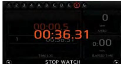
1. With the STOP WATCH screen displayed, push <START/STOP>. The timer-on indicator will flash when the stopwatch function is active.
