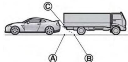
The position **(C)** is shown further than the position **(B)** in the display. However, the position **(C)** is actually at the same distance as the position **(A)**. The vehicle may hit the object when backing up to the position **(A)** if
