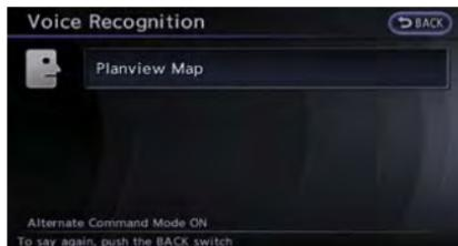
4. Voice feedback will be provided when the command is accepted, and the map is displayed in 2D (Plan View).
