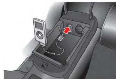
Open the console lid and connect the iPod® cable to the USB connector. If the iPod® supports charging via USB, the battery of the iPod® will be charged while connected to the vehicle.
