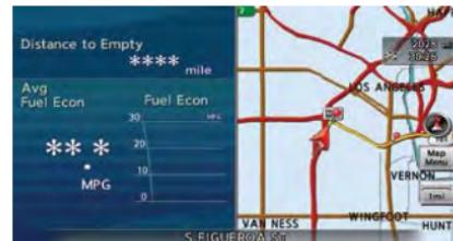
The current fuel consumption rate, average fuel consumption rate, instantaneous consumption rate and distance to empty can be displayed on the map screen. An enlarged intersection view is automatically displayed when the vehicle approaches the guide point.
