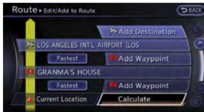
7. By highlighting [Calculate] and pushing **<ENTER>**, the system will recalculate the routes. After the route search is completed, the display will automatically return to the current location map screen.
