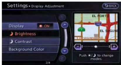
Adjust the display brightness by rotating the center dial in the direction of [+] or [-].
