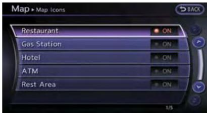
3. Highlight the preferred icon and push **<ENTER>**. The icon display setting toggles between on and off each time **<ENTER>** is pushed. The indicator of the selected icon illuminates.
