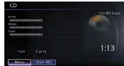
Push the ignition switch to the ACC or ON position and insert the Compact Disc (CD) into the slot with the label side facing up. The CD will be guided automatically into the slot and start playing.
