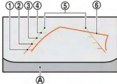
Guiding lines which indicate the vehicle width and distances to objects with reference to the bumper line **(A)** are displayed on the monitor.
