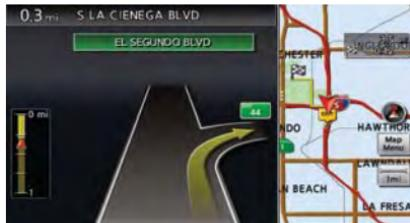
While driving on a freeway, when the vehicle is approximately 1 mile (approximately 2 km) from a junction, the system automatically switches to the split screen and displays an enlarged view of the junction (3D) on the left screen. After passing the junction, the system automatically returns to the full screen mode. To switch to the full screen mode while the enlarged junction view is displayed, push **<MAP>**. Pushing **<MAP>** again displays the enlarged junction view.
