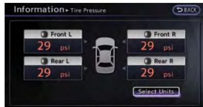
The pressure indication “\*\* psi” on the screen means that the tire pressure is being measured. After a few driving trips, the pressure for each tire will be displayed.
