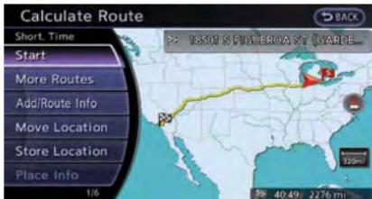
4. The entire route to the home location is shown on the map. Highlight [Start] after confirming the location of the displayed destination, and push <ENTER>. The system sets the destination to the selected location and starts calculating a route.
