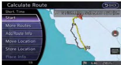
8. The entire route is shown on the map. Highlight [Start] after confirming the location of the displayed destination, and push **<ENTER>**. The system sets the destination to the selected location and starts calculating a route.
