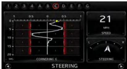
Displays the steering angle, vehicle speed and the g-force being exerted on the vehicle.
