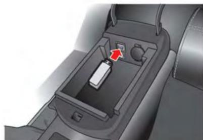
Open the console lid and connect a USB memory as illustrated. Then, push **<DISC-AUX>** repeatedly to switch to the USB memory mode.
