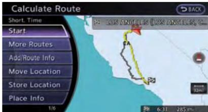
6. The selected destination is displayed at the center of the map. Highlight [Start] after confirming the location of the displayed destination, and push <ENTER>.
