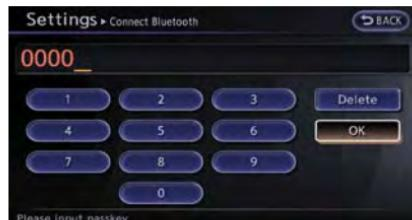
4. Choose a PIN code to use with the compatible Bluetooth® audio device using the number input screen. The PIN code will need to be entered into the Bluetooth® audio device after step 5. Select [OK].
