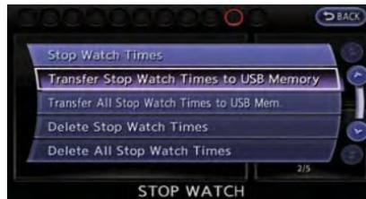
4. Select [Transfer Stop Watch Times to USB Memory]. The time record is saved to the USB memory.
