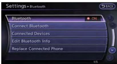
To set up the Bluetooth® device system to the preferred settings, push **<SETTING>** and select [Bluetooth].
