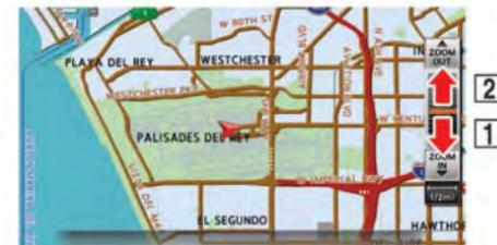
1. Turn the center dial when the map screen is displayed. The map scale is displayed at the right side of the screen.
