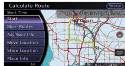
9. The entire route is shown on the map. Highlight [Start] after confirming the location of the displayed destination and push <ENTER>. The system sets the destination to the selected location and starts calculating a route.
