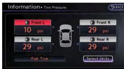
If the system detects a puncture, the punctured tire is displayed in red, and a warning message appears.
