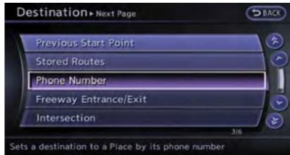
3. Highlight [Phone Number] and push <ENTER>. The telephone number input screen is displayed.
