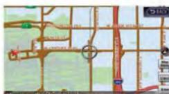
The basic map screen displays the current location (the position where the vehicle mark is located). Push <MAP> to display the current location on the map while on any screen.
