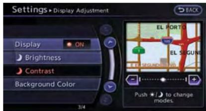
Adjust the display contrast by rotating the center dial in the direction of [+] or [-].
