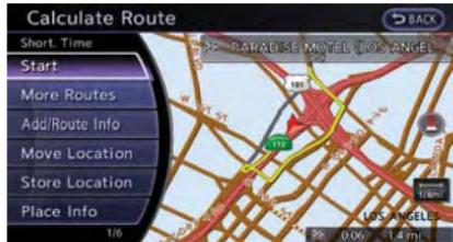
5. The entire route is shown on the map. Highlight [Start] after confirming the location of the displayed destination, and push **<ENTER>**. The system sets the destination to the selected location and starts calculating a route.
