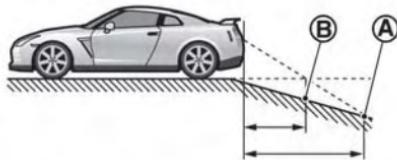
When backing up the vehicle down a hill, the distance guide lines and the vehicle width guide lines are shown further than the actual distance. For example, the display shows 3 ft (1.0 m) to the place **(A)**, but the actual 1.0 m (3 ft)
