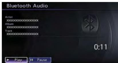
Push the ignition switch to the ACC or ON position. Then, push **<DISC-AUX>** repeatedly to switch to the Bluetooth® audio mode. If the system has been turned off while the Bluetooth® audio device was playing, pushing the ON-OFF/VOL control knob will start the Bluetooth® audio device.
