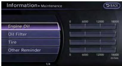
To set the maintenance interval for the engine oil, oil filter, tire and other reminders, choose an item and push **<ENTER>**.
