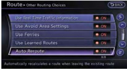
4. Highlight [Auto Reroute] and push <ENTER>. The indicator illuminates. When the current location map screen or route setting screen is displayed, the system recalculates a route with the set conditions.
