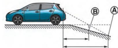
When moving the vehicle down a hill, the distance guide lines and the vehicle width guide lines are shown further than the actual distance. For example, the display shows 3 ft (1 m) to the place ①, but the actual 3 ft (1 m) distance on the hill is the place ②. Note that any object on the hill is viewed in the monitor closer than it
