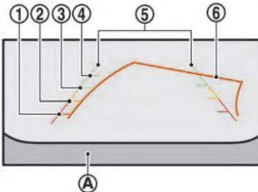
wheel is turned. The predictive course lines will move depending on how much the steering wheel is turned and will not be displayed while the steering wheel is in the neutral position.
