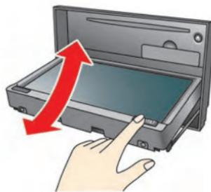
Open the monitor to insert/eject a CD or an SD card.
