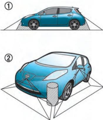
There are some areas where the system will not detect objects. When in the front or the rear view display, an object below the bumper or on the ground may not be detected ①. When in the bird's-eye view, a tall object near the seam of the camera detecting areas will not appear in the monitor ②.
