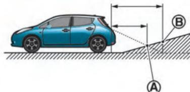
When moving the vehicle up a hill, the distance guide lines and the vehicle width guide lines are shown closer than the actual distance. For example, the display shows 3 ft (1 m) to the place ①, but the actual 3 ft (1 m) distance on the hill is the place ②. Note that any object on the hill is viewed in the monitor further than it
