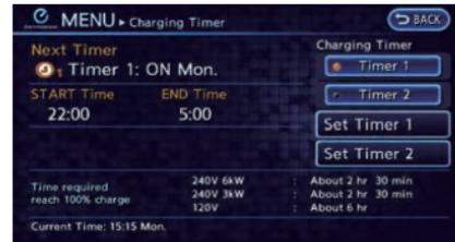
Charging of the Li-ion battery will automatically start at a scheduled time according to the start time, end time and day of the week set. The timer charge function allows two different timer settings. Each timer charge can be set to activate on a different day of the week. If no timer is set, the charge will start immediately after connecting the charge connector.
