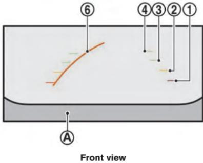
Guiding lines, which indicate the vehicle width and distances to objects with reference to the vehicle body line **(A)**, are displayed on the monitor.
