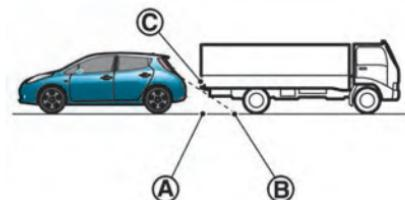
The position **(C)** is shown further than the position **(B)** in the display. However, the position **(C)** is actually at the same distance as the position **(A)**. The vehicle may hit the object when moving toward the position **(A)** if the object projects over the actual moving course.
