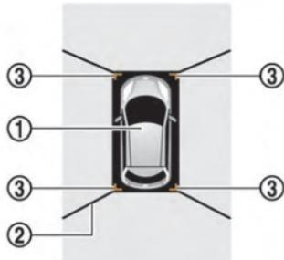
The bird's-eye view shows the overhead view of the vehicle which helps confirm the vehicle position and the predictive course to a parking space.
