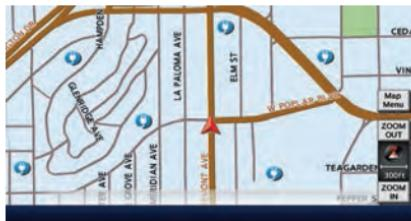
Icons for charging stations can be displayed on the map. You can also display only charging stations that are equipped with quick charge devices or only charging stations that are equipped with normal charge devices.
