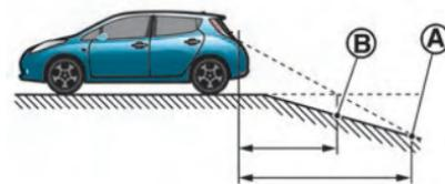
When backing up the vehicle up a hill, the distance guide lines and the vehicle width guide lines are shown closer than the actual distance. For example, the display shows 3 ft (1 m) to the place **(A)**, but the actual 3 ft (1 m) distance on the hill is to the place **(B)**. Note that any object on the hill is further than it appears on the
