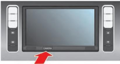
When you push the **CAMERA** button or shift the shift lever into the "R" (Reverse) position while the power switch is in the ON position, the Around View Monitor operates. The monitor displays various views of the position of the vehicle.
