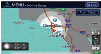
By pressing the
