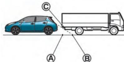
The position (C) is shown further than the position (B) in the display. However, the position (C) is actually at the same distance as the position (A). The vehicle may hit the object when backing up to the position (A) if the object projects over the actual backing up course.
