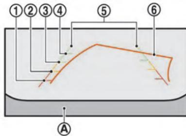
Guiding lines which indicate the vehicle width and distances to objects with reference to the bumper line (A) are displayed on the monitor.
