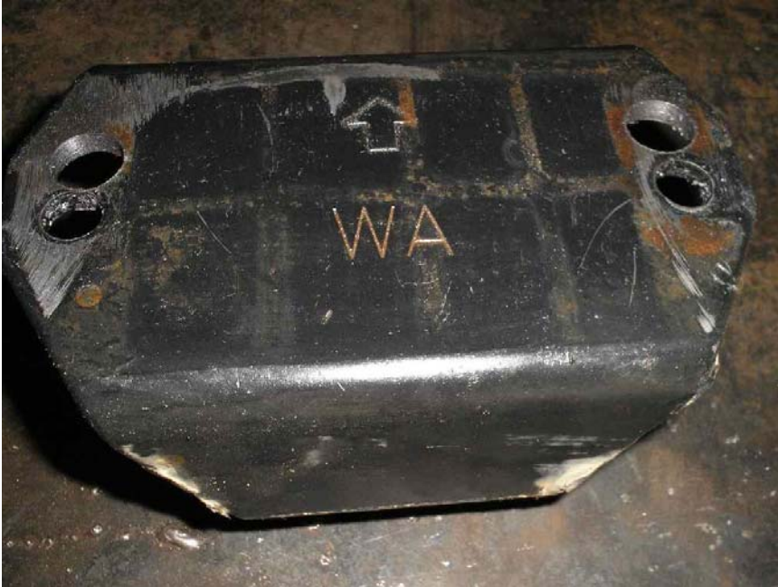
Fig. 4.8 Automatic Transmission motor mount red-drilled for Manual Transmission.
