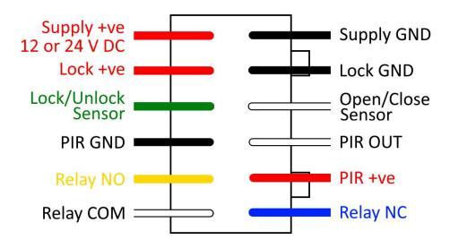
Here's the pinout of the connector which is used for this controller. The above schematic as viewed from the tail end of the connector, with the wires split along the center. Label all the necessary wires needed to interface with your lock before proceeding.
