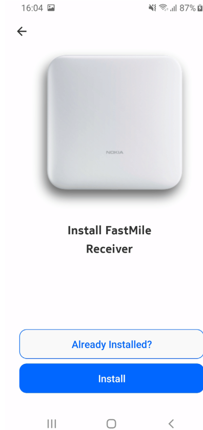
Figure 25 Screen showing the Already Installed option for unit managed by the Nokia Altiplano FastMile Controller through NETCONF
