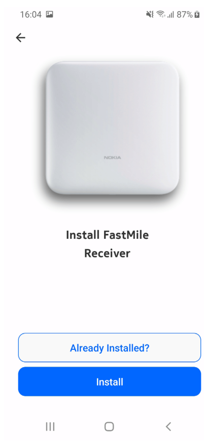
Figure 42 Screen showing the Already Installed option for unit managed by an ACS through TR-069
