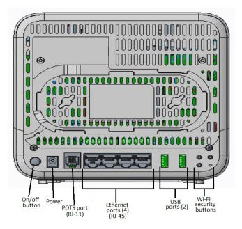
**<sup>3</sup>** Power down the unit by using the on/off power switch.
