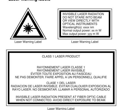
*Figure 12* Laser warning labels
