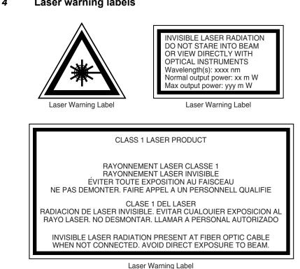
*Figure 4* Laser warning labels
