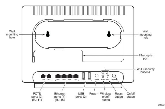
Figure 11 shows the G-240W-G ONT without the fiber cover.
