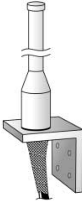
Properly weatherproofed antenna connection. Antenna mounting brackets may vary.
