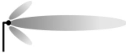
Directional Antennas - Radiation Pattern Side View
