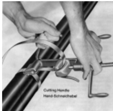
Fig. 2.14. Cutting the band
