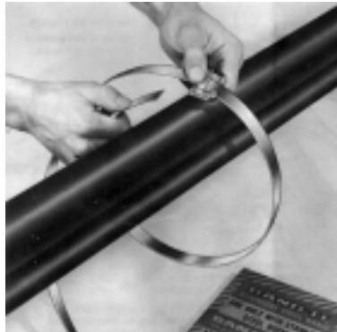
Fig. 3.7. Buckle slided on band
