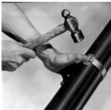
Fig. 2.16. Hammering buckle ears
