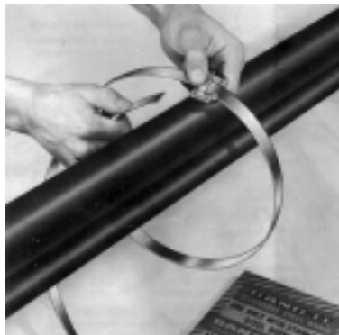
Fig. 2.9. Buckle slided on band
