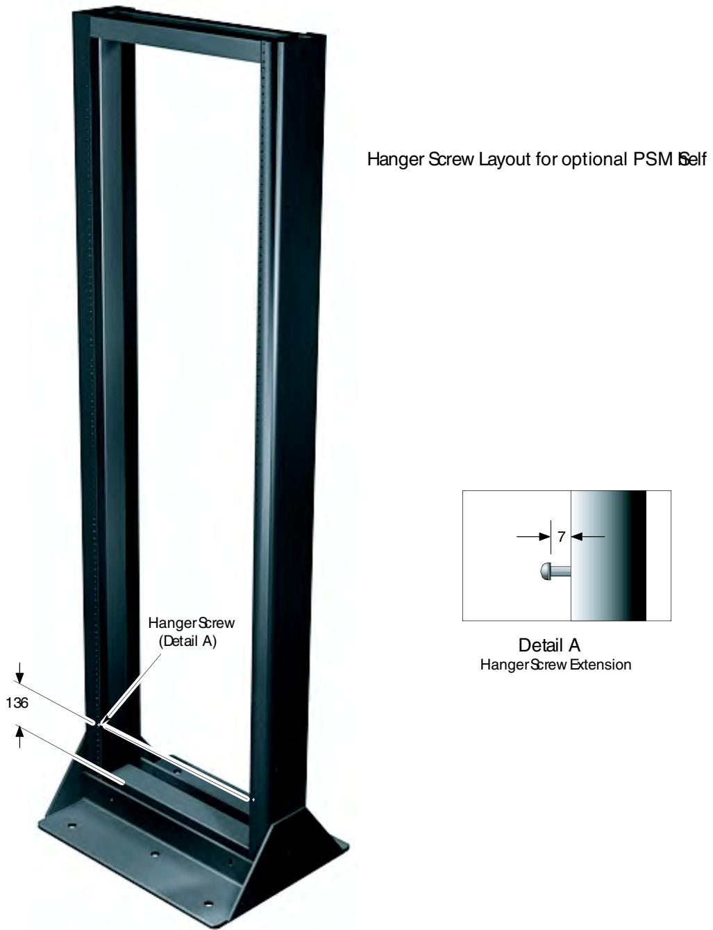
Figure 2-13 Hanger screw layout for the optional PSM shelf
