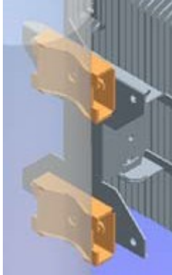
Figure 3-4 Wall-mount bracket to pole-mount bracket
