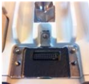
Figure 2-4 9764 MCO Wi-Fi AP connection point on 9764 MCO
