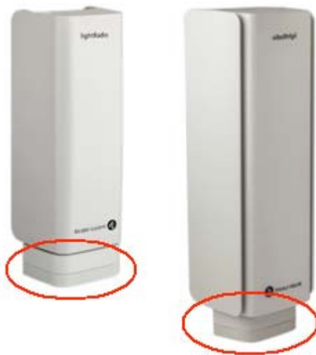
Figure 2-1 9764 MCO Wi-Fi AP attached to 9764 MCO hardware variants
