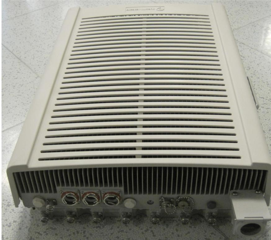
Figure 5 -B41 RRH8x20-B with solar shield
