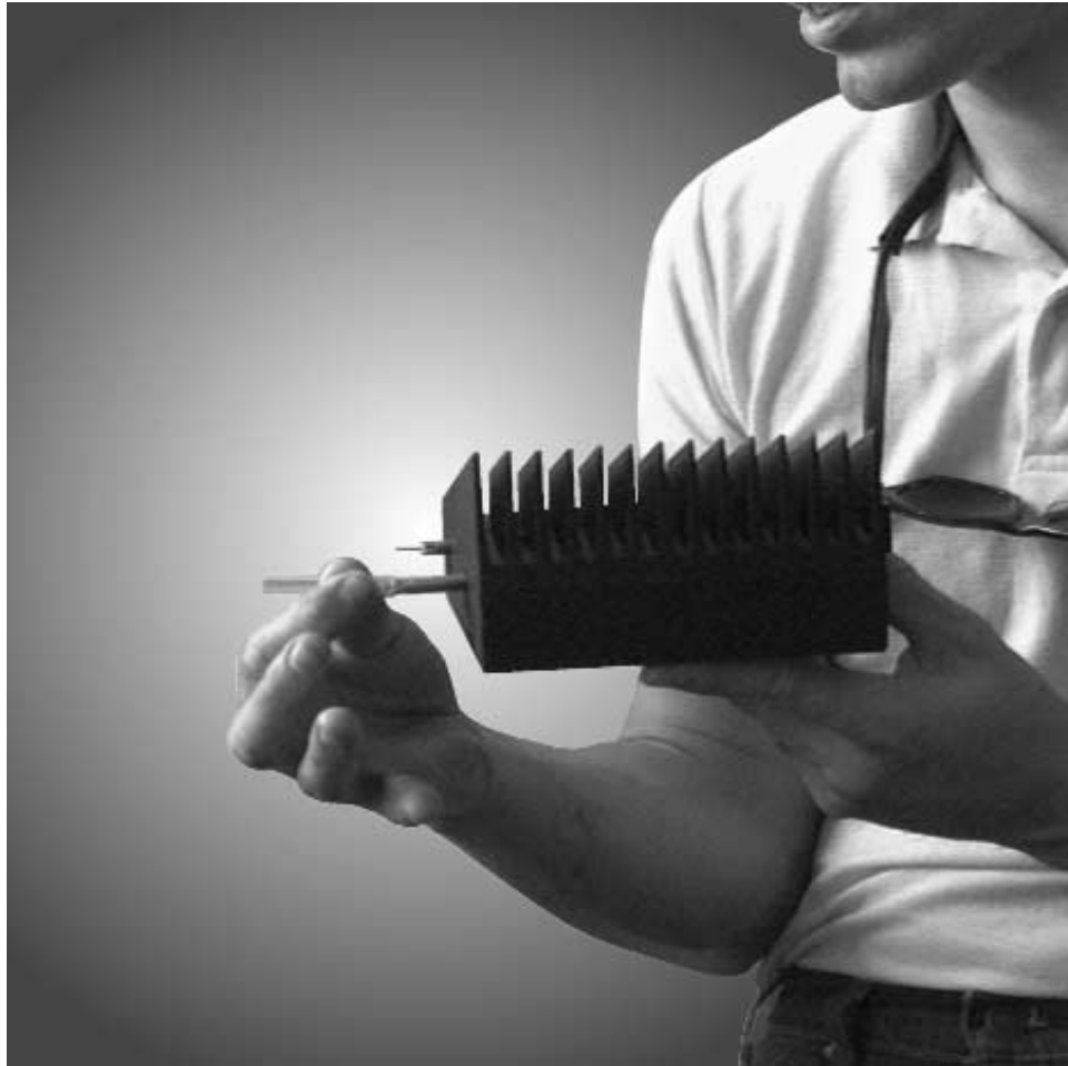
Figure 22-20. RF connectors on each LAM
