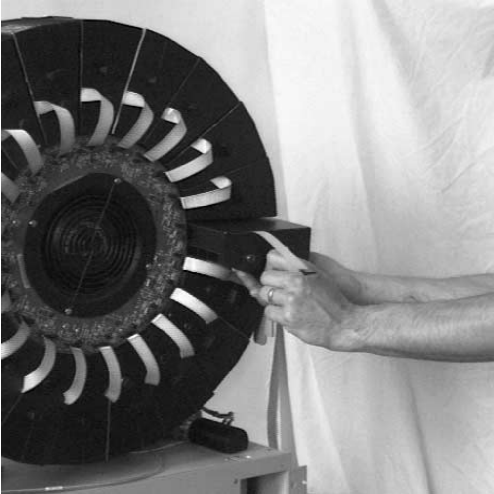
Figure 22-19. Unscrew the LAM from its standoff
