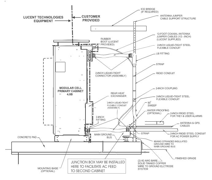
NOTE: THE SOUND MUFFLER MOUNTED ON THE REAR OF THE CABINET IS NOT ILLUSTRATED IN THIS VIEW. IT IS PART OF THE LUCENT EQUIPMENT
