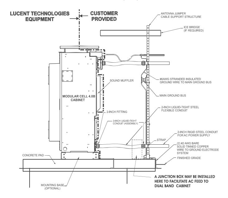
NOTE: THE OPTIONAL REAR HEAT EXCHANGER IS NOT ILLUSTRATED IN THIS VIEW. IT IS PART OF THE LUCENT EQUIPMENT
