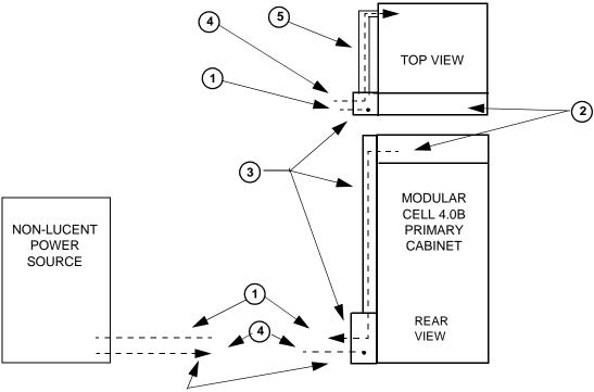
If the power source is not flush mounted with zero spacing to the cable duct, a 2-inch conduit is used for routing of cables between the cable duct. and the non-Lucent power source
