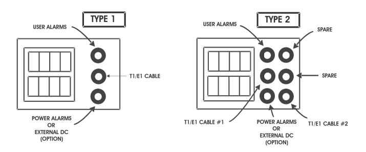
**6** Allow a minimum of 2 meters (6.5 feet) of the alarm cable for routing inside of the Modular Cell 4.0B primary cabinet and cut off the remainder.
