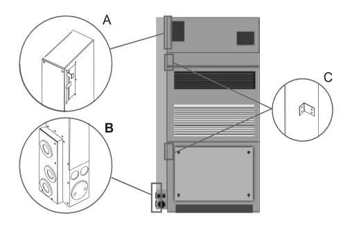
**Detail A:** Connections for six hex-head screws
