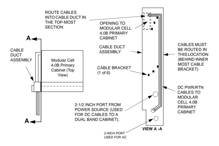
5 If the DC cables need to be shortened before they are attached in the non-Lucent power source, the labels may be cut off. Remember to relabel each cable immediately after it is cut.
