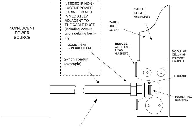
If flush mounting is not possible, conduit (example) should be used for routing of cables from the non-Lucent power source to the cable duct.
