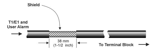
**Important!** When performing the next step, take care not to insert the cable insulation (above the stripped area) more than 3/8-inch into the rubber strain relief insert.
