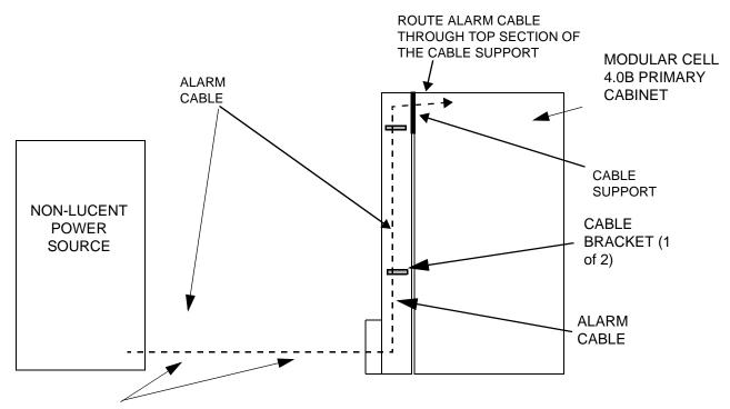
If flush mounting is not possible, two 2-inch conduit s are used for routing of cables from the non-Lucent power source to the cable duct. The middle (upper 2-inch) conduit is used to route the power alarm cable **Important!** When performing the next step, keep the alarm cable in the top section of the opening in the cable duct.
