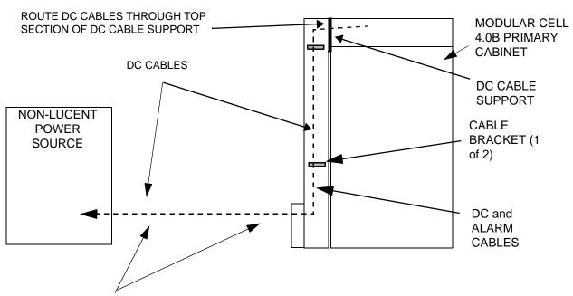
If the power source is not flush mounted to the cable duct, conduits are used for routing of cables from the non-Lucent power source to the cable duct.
