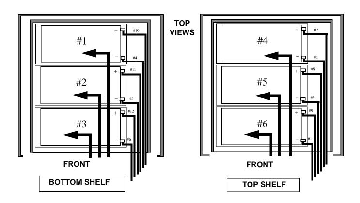
2 Insert the previously removed top portion of the battery retaining brackets as a spacer on the right side of the batteries as shown below.
