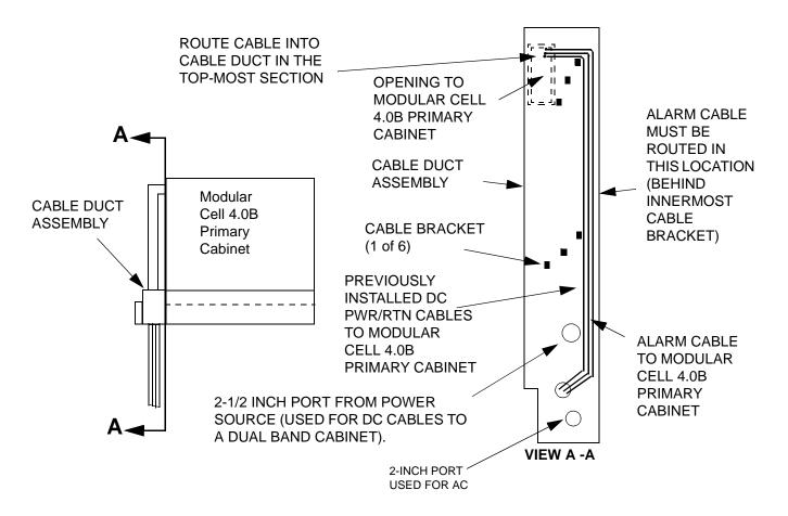
Route the cable out the top of the duct and to the alarm cable entry point on the top rear of Modular Cell 4.0B. Refer to the figure below for the location of the alarm cable entry point in the two types of feed-through configurations that may be encountered
