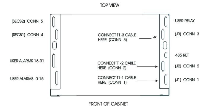
The figure below shows the cable termination points on the Integrated Power Module bracket located on top of the Integrated Power Module and is for the Digital Only with two Digital Shelves version of the BTS 8420/AWS 8420 radio cabinet. It is only for configurations with integrated power. Again, only callouts for T1 cable connections are shown here. The bracket will have labels that match one of the figures below.
