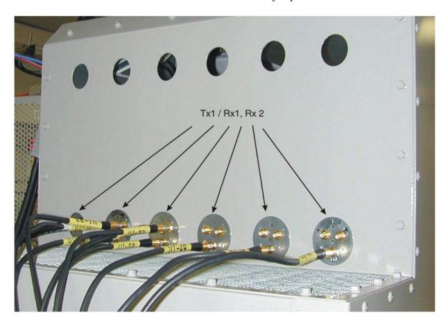
Shown in the figure below are the RF antenna jumper cable interface connectors on the rear panel of the *Filtered* and *Low Power* versions equipped with 850 MHz and 1900 MHz filters.
