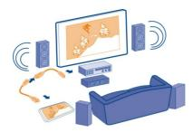
Connect the HDMI adapter to the HDMI connector of your phone.
