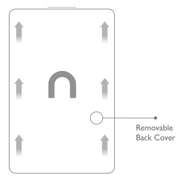
Do not press on the middle of the back cover or bend your NOOK. Doing so might damage the screens.
