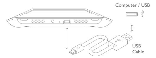
When you connect your NOOK to a personal computer using USB, it enters USB drive mode and charges. If you want to charge your NOOK and use it (as opposed to using USB drive mode), eject/unmount the NOOK drive (and the drive for a supplemental microSD card if present), but leave your NOOK plugged into the USB port on your computer.
