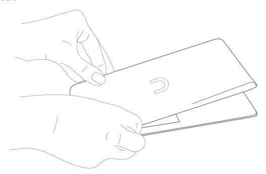
Moving your hands up the edges of the back cover (where the raised parts of the back are), press down gently in the places shown. You should hear snapping sounds.
