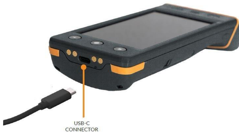
Picture 3 Charging of the Nordic ID HH83 via USB charger
