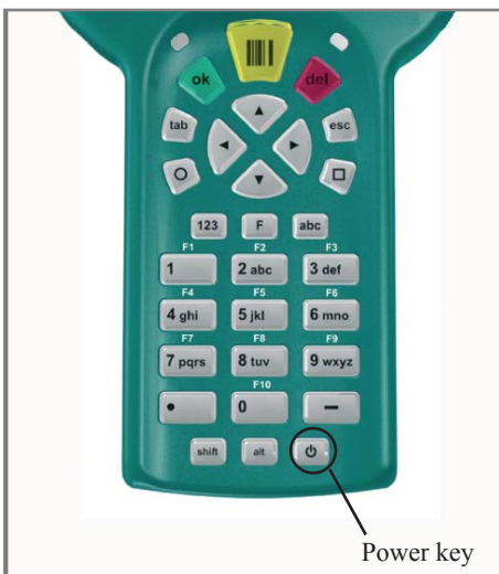
Fig.19 Switching on the power
