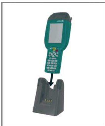
Fig.15 Placing the PL3000 to the charger
