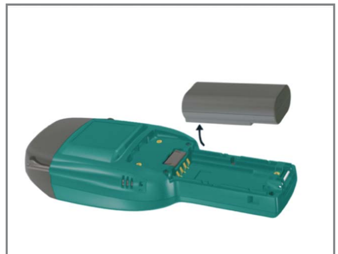
Fig.4 Removing the battery
