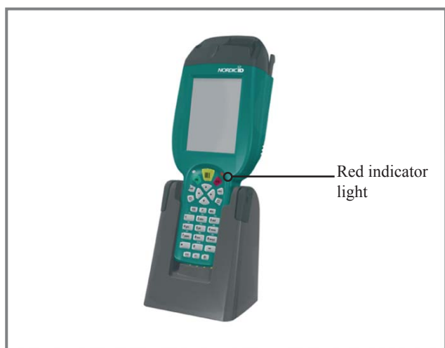
Fig.16 Red indicator light shows that battery has less than 90% of the capacity
