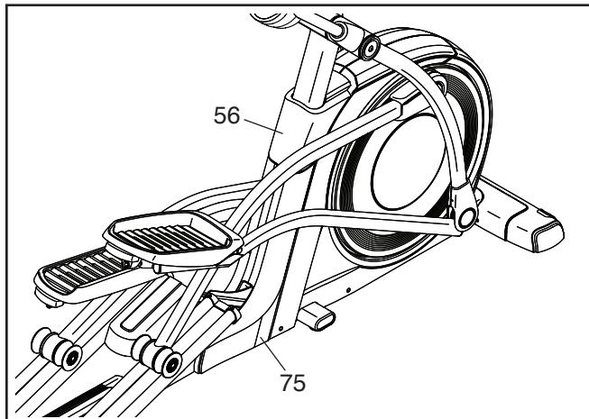
Then, remove the four M4 x 16mm Screws (not shown) from the upper and lower ends of the Rear Shield (75), and remove the Rear Shield.
