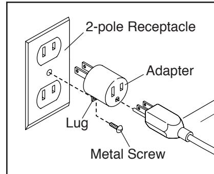
The lug or wire extending from the adapter must be connected with a metal screw to a permanent ground such as a properly grounded outlet box cover. Some 2-pole receptacle outlet box covers are not grounded. Before using an adapter, contact a qualified electrician to determine whether the outlet box cover is grounded before using an adapter. The temporary adapter should be used only until a properly grounded outlet can be installed by a qualified electrician.
