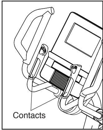
Be careful not to move your hands excessively or to squeeze the contacts tightly. For optimal performance, clean the contacts using a soft cloth; **never use alcohol, abrasives, or chemicals to clean the contacts.**
