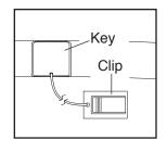
gency, the key can be pulled from the console, causing the walking belt to slow to a stop. Test the clip by carefully taking a few steps backward; if the key is not pulled from the console, adjust the position of the clip.
