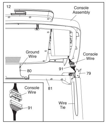
Set the console assembly on the Left and Right Handrails (79, 83). Make sure that no wires are pinched. Insert the excess Upright Wire (91) behind the Console Frame (101).
