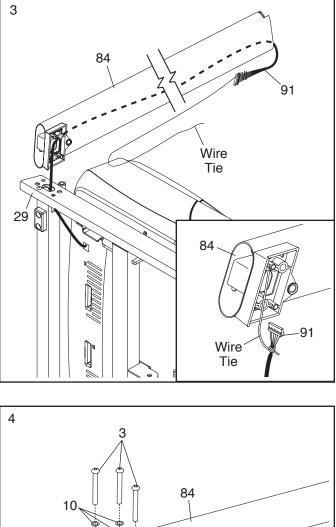
4. With the help of a second person, hold the Left Upright (84) against the Base (29). Be careful not to pinch the wires. Partially tighten three 3/8" x 4" Screws (3) with three 3/8" Star Washers (10) into the Left Upright and the Base; do not fully tighten the Screws yet.
