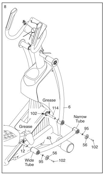
Identify the Right Upper Body Arm (8), which is marked with a "Right" sticker, and orient it as shown.
