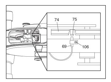
Next, loosen, but do not remove, the indicated M4 x 16mm Screw (106). Slide the Reed Switch (69) slightly toward or away from the Pulley Magnet (75). Then, retighten the M4 x 16mm Screw.
