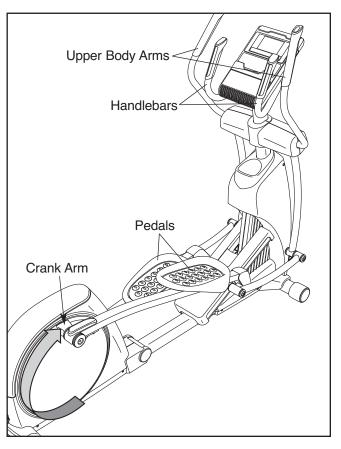
Note: The crank arms can turn in either direction. It is recommended that you turn the crank arms in the direction shown by the arrow; however, for variety you can turn the crank arms in the opposite direction.
