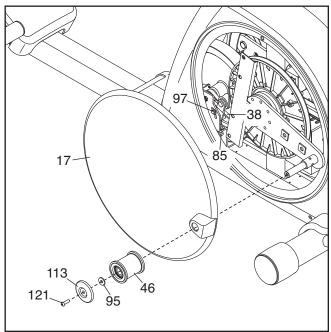
Next, loosen the Pivot Screw (97). Tighten the Belt Adjustment Screw (85) until the Drive Belt (38) is tight. When the Drive Belt is tight, tighten the Pivot Screw.
