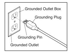
current to reduce the risk of electric shock. This product is equipped with a cord having an equipment-grounding conductor and a grounding plug. Plug the power cord into an appropriate outlet that is properly installed and grounded in accordance with all local codes and ordinances. This product is for use on a nominal 120-volt circuit. Important: The elliptical exerciser is not compatible with GFCI-equipped outlets.
