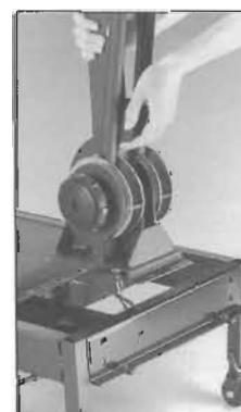
Figure 9 Position the upper-body exerciser over the treadmill base. Insert the resistance cable and sensor cord through the opening in the treadmill base.
