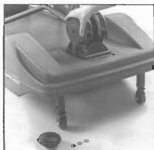
Figure 4 Remove the parts in the following order: upper-body resistance knob, washer, bearing, washer, right brake-pad plate.
