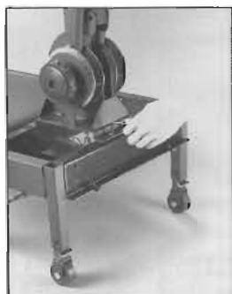
Figure 10 Use the 3/16-inch Allen wrench to tighten the bolts that secure the upper-body exerciser to the treadmill base.
