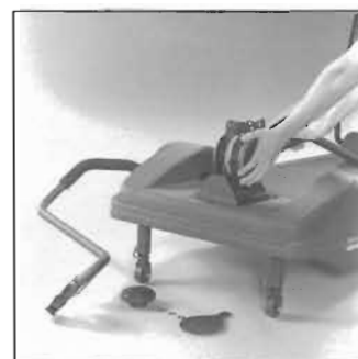
Figure 5 Remove the left arm-exerciser pole, the left brake-pad plate and the large bolt. The upright tube will slide out of position as you do this.
