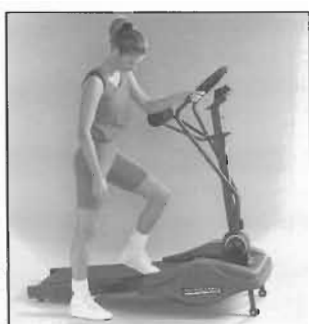
Figure 9 Use your foot to spin the treadmill belt for several revolutions. This will help to center the treadmill belt on the treadmill deck.
