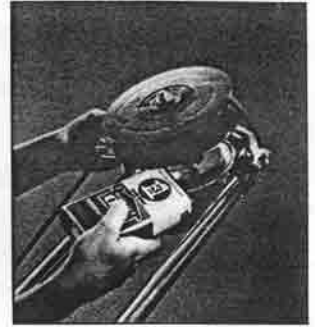
Figure 2: After lifting the cord drum assembly for the 350, 450 and World Class, roughen the surface of the brake pad with an emery cloth or file. Then place a few drops of light household oil on the pad.
