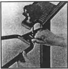
Figure 3: Insert the easy-lock pin through the holes, and rotate it over the right side of the hip-pad bracket.
