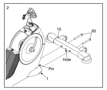
While a second person lifts the rear of the Frame (1), attach the Rear Stabilizer (16) to the Frame with two M10 x 105mm Screws (65).
