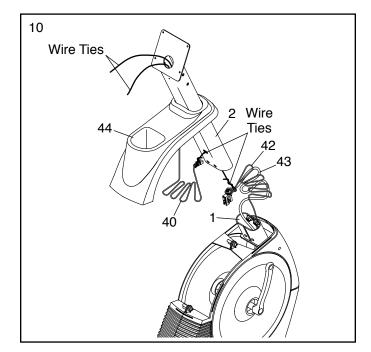
11. **Tip: Avoid pinching the wires.** Slide the Upright (2) onto the Frame (1).
