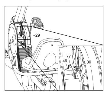
Then, retighten the M4 x 16mm Screw (77). Plug in the power adapter and turn the Pulley (29) for a moment. Repeat these actions until the console displays correct feedback.
