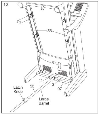
11. Attach the upper end of the Storage Latch (53) to the Frame (56) with a 3/8" x 1 3/4" Bolt (6) and a 3/8" Nut (11). Note: It may be necessary to move the Frame (56) back and forth to align the Storage Latch with the Frame.
