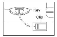
console. Note: It may take a minute for the console to be ready for use. IMPORTANT: In an emergency, the key can be pulled from the console, causing the walking belt to slow to a stop. Test the clip by carefully taking a few steps backward; if the key is not pulled from the console, adjust the position of the clip.
