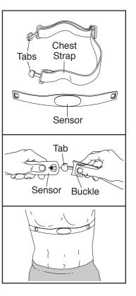
side-up. Then, attach the other end of the chest strap to the sensor. Adjust the length of the chest strap, if necessary.
