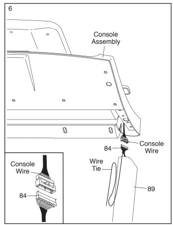
Insert the wires into the Left Upright (89) as you set the console assembly on the Left Upright and the Right Upright (90). Be careful not to pinch the Upright Wire (84).
