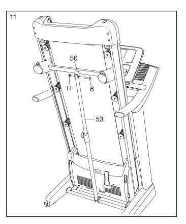
12. Remove the packaging material from the bottom of the Frame (56).
