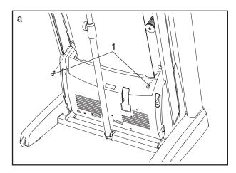
Lower the treadmill (see HOW TO LOWER THE TREADMILL FOR USE on page 27). Remove the three #8 x 3/4" Screws (1). Carefully pivot the Motor Hood (71) off.
