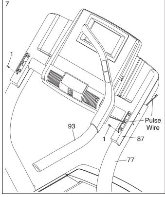
8. Set the Right Handrail Assembly (93) onto the right Upright (77). Make sure that no wires are pinched.
