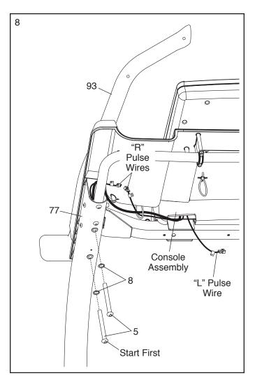
8. Hold the Left Handrail Assembly (86) near the left Upright (77). Insert the pulse wire from the left handrail assembly into the hole in the top of the Upright and pull it out of the end of the Upright.
